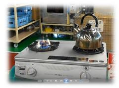
Using Natural Gas Burner with pure LPG (Propane)
