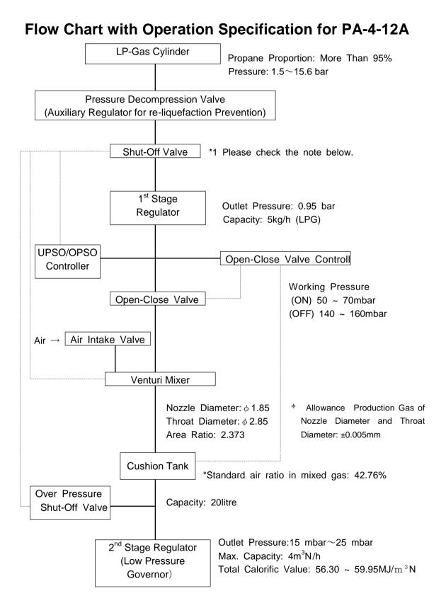
\*1 Working Pressure for Shut-Off Valve
