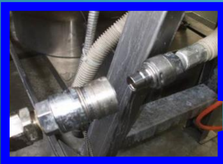
Quick fitting is able to be disconnected without tools.
