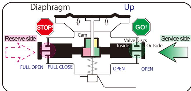
When there is higher inlet pressure on the supply side, this lifts the diaphragm and partially opens both the inside and outside valve discs.
