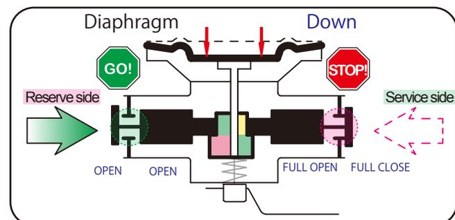
As the liquid in the service side decreases this leads to lower pressure and the diaphragm drops, this will lead to the outside disc on the service side fully closing and cuts off the liquid supply.
