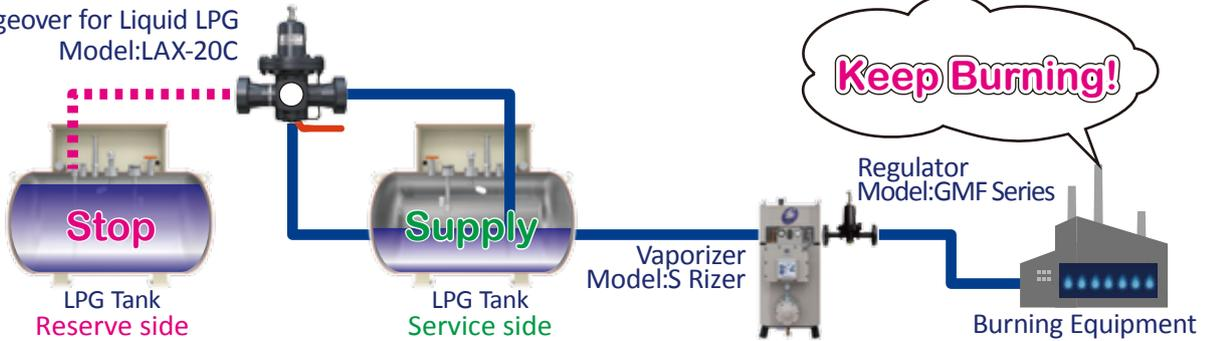
Use this valve in conjunction with cylinders/tanks supply though a Vaporizer.
